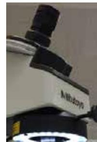
The adjustable LED circular illumination provides more than twice the intensity of the standard oblique surface illumination system and mounts easily to the OD of the objective lens.
